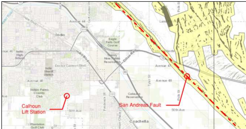
Calhoun Lift Station Fault Sources
