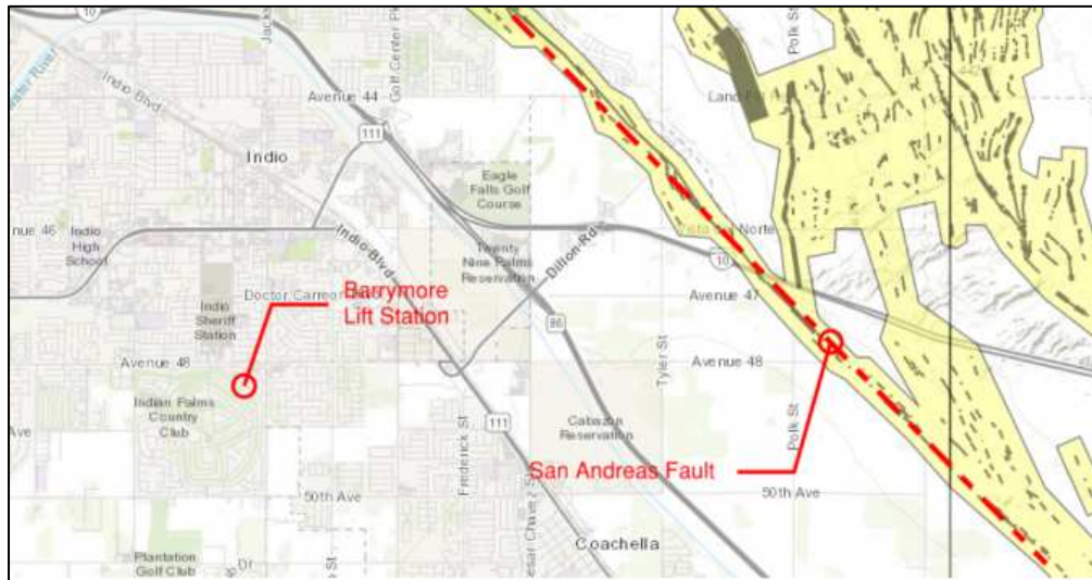
Barrymore Lift Station Fault Sources
