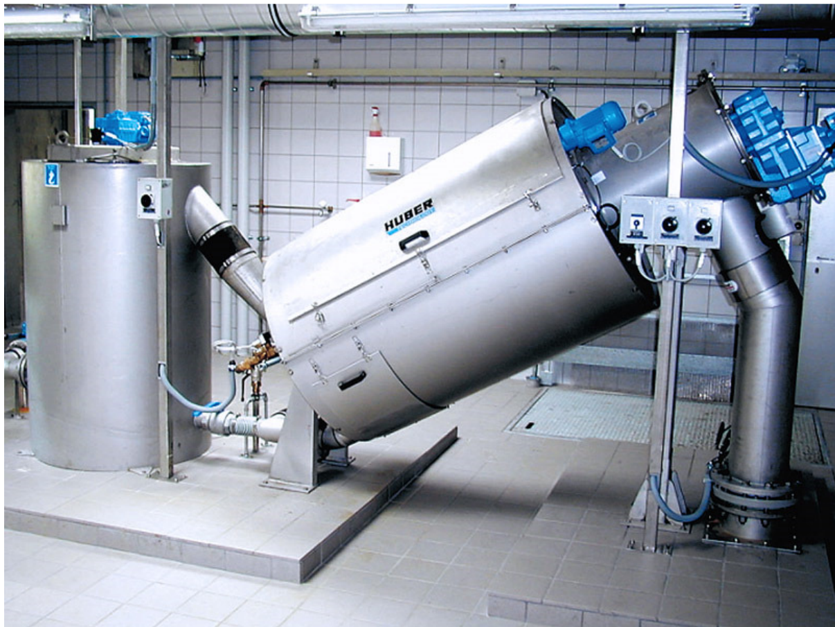
Figure 3 Example of an Installed Rotary Drum Thickener (by Huber)
